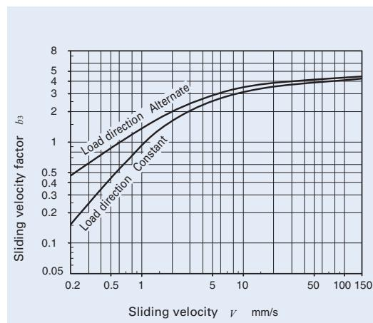
Fig. 4 Sliding velocity factor for lubrication type PILLOBALLS
